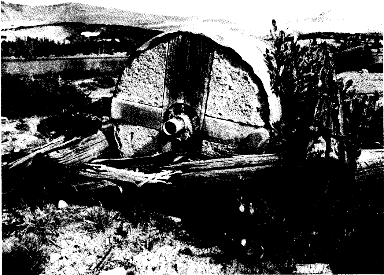
This stock-drawn roller with log tongue was used to compact and grade earth-fill. The roller was constructed on-site at Five Point Lake Dam.
