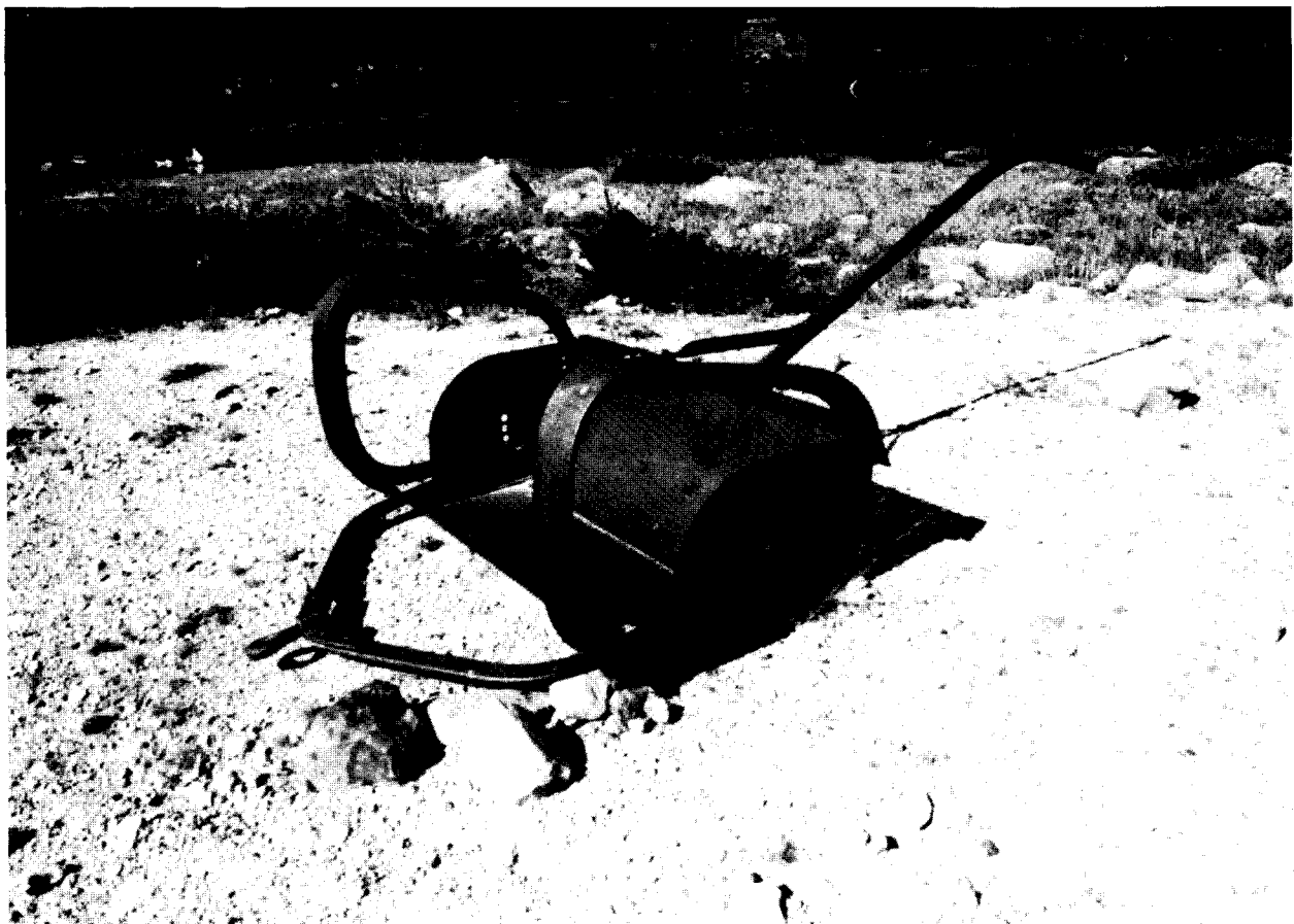
Steel, team-drawn earth scrapers such as this one left behind at Five Point Lake Dam removed and hauled earth-fill to dam sites.
