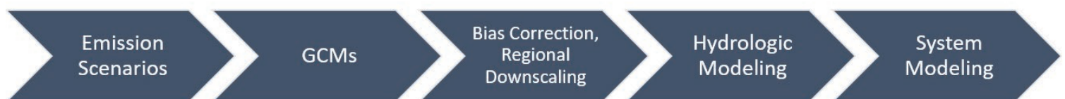
Figure 16. General processing steps from GCMs to basin-scale hydrology and water planning.
