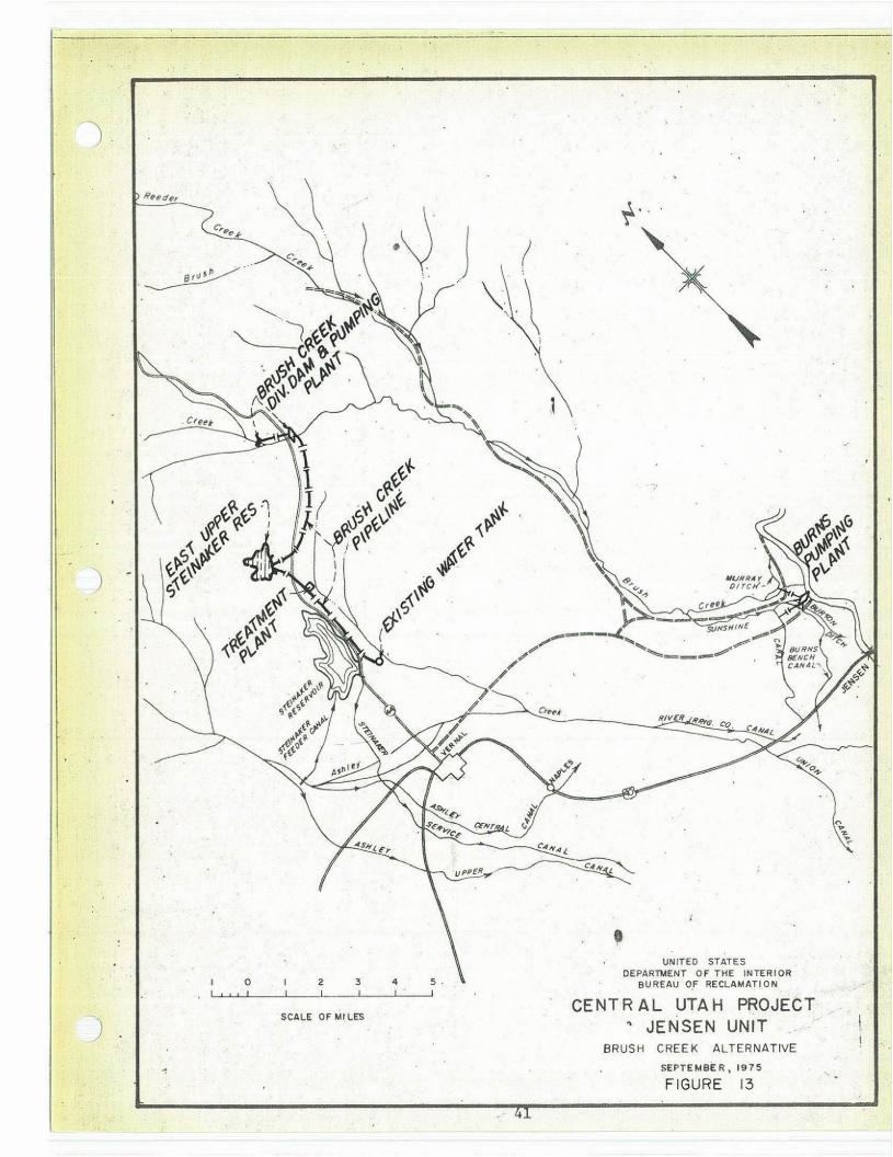
the average annual yield of Tyzack Reservoir by 5,100 acre-feet. This would also result in a reduction in size of the Burns Pumping Plant to 86.7 second-feet.
