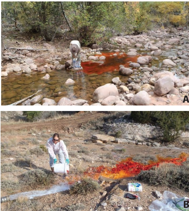
Figure 15. Melissa Hendrickson injecting the dye for the (A) first and (B) second dye tests. The protective clothing in B was to prevent contamination from windblown powdered dye.
