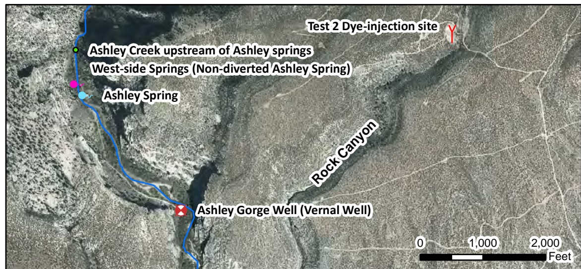
Figure 12. Locations of dye pour sites and dye monitoring sample collection for dye tracer tests conducted in this study.
